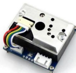
Figure 2 Physical diagram of GP2Y1010AU0F sensor
